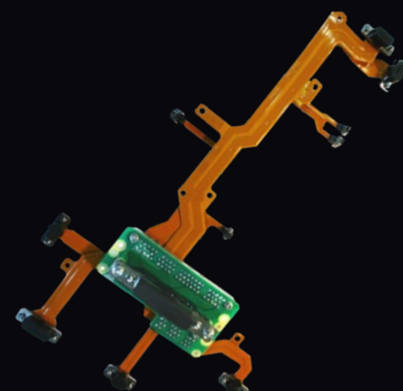
Production flex and rigid flex assembly terminated, tested and ready for immediate use
