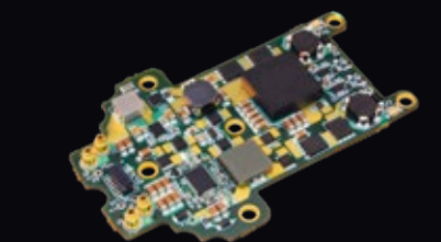
Ruggedized power distribution PCBA for use in STAR-PAN™ soldier system
