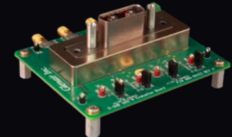
HiPer-D connector with size #8 opto-electronic contacts evaluation board
