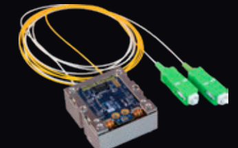
PCBA design for radio frequency-over-fiber links for SATCOM and RF signal distribution
