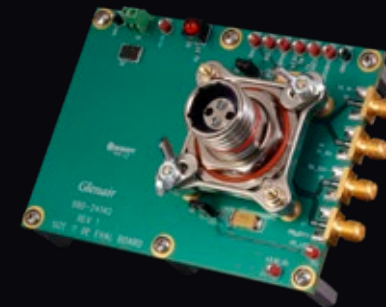
MIL-DTL-38999 type 2.5mm ELIO® compatible transceiver evaluation board
